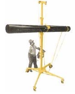
This dependable lift can raise a 682 kg load to heights up to 7.6 m in minutes. In addition, the load can be moved vertically and horizontally at the same time. Wider loads can be handled with the addition of the Tee Head Extension Bar. The Roust-A-Bout eliminates the need for many other tools such as come alongs, scaffolds, monorails, and swing booms.
