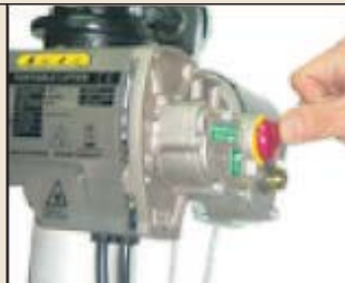
Emergency Stop Button
