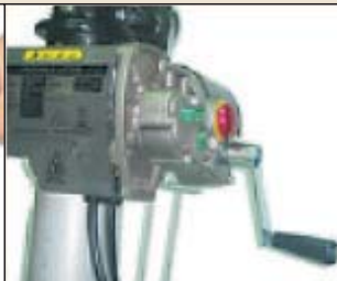
Manually Manual controls available in case of a power failure
