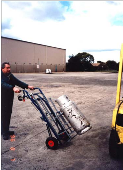
Wheel up to Gas Bottle and attach to cradle using cradle strap.
