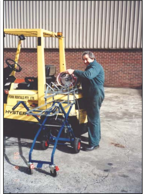
Position FlexiLifter adjacent to forklift, lock castors, undo bottle strap & slide gas bottle into position onto forklift.
